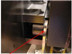
Adjust front cam followers so front pusher dogs are pushing 100 % of pallet edge. The rear cams are adjusted so rear dogs are pushing 90 % of pallet edge.
